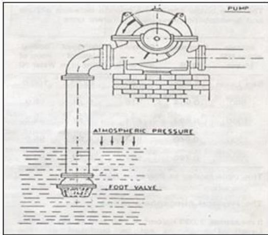
**Fig. 6:** Priming by foot valve
