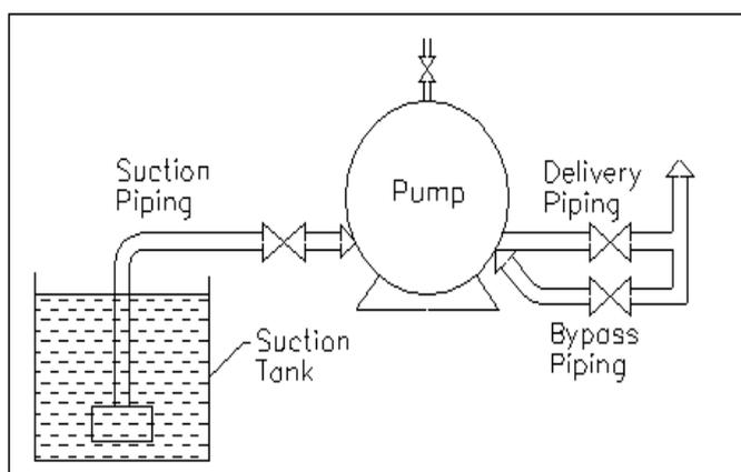
**Fig. 4:** Priming with bypass around the discharge check valve
