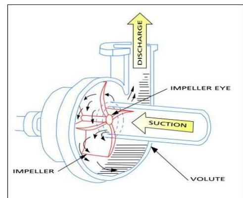
Fig.1: Centrifugal pumps
