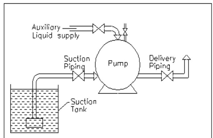
**Fig. 5:** Priming by foot valve with auxiliary liquid supply
