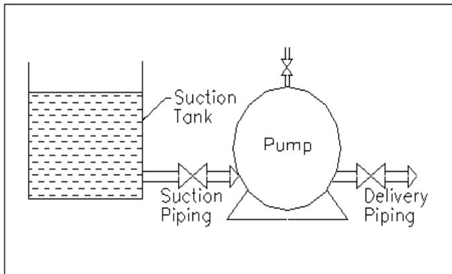
**Fig.3:**Priming with flooded suction
